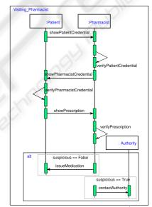
Figure 4: UML Sequence Diagram representing the "Visiting a pharmacist" system requirements.
