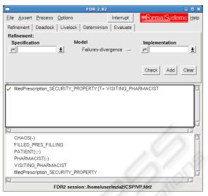
Figure 6: An FDR2. screenshot, reflecting the successful check of a security requirement. Here, *FILLED\_PRES\_FILLING* is the specification process, *filled-Prescription\_SECURITY\_PROPERTY* is the security assertion, and the remaining are implementation processes.
