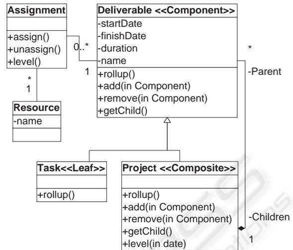
Figure 1: UML class diagram illustrating the WBS hierarchy.
