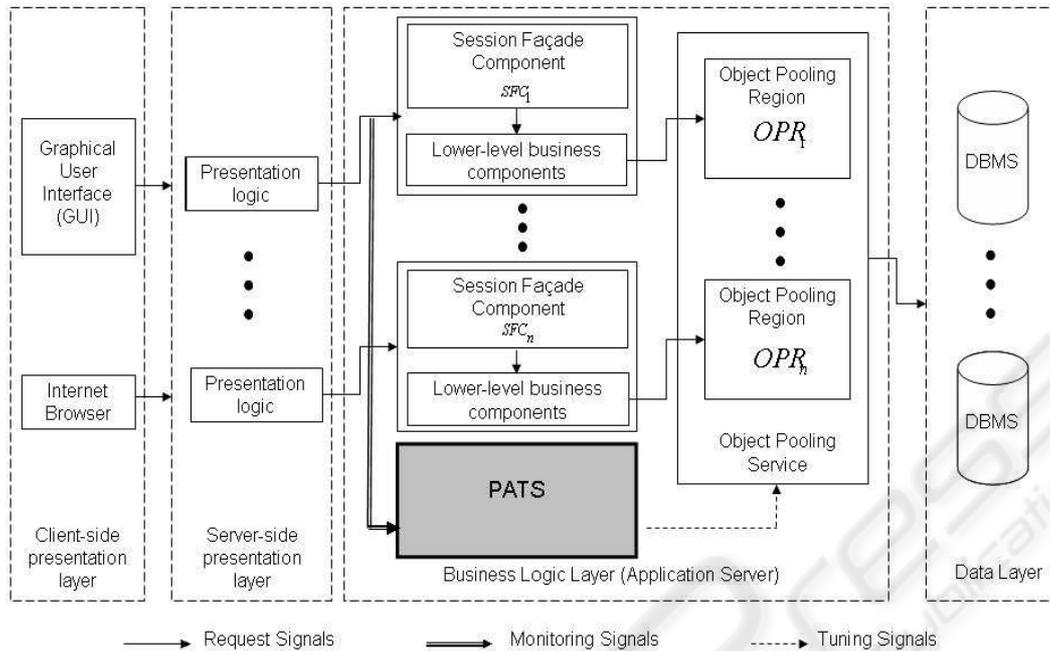
Figure 1: Integration of PATS into the middleware-based enterprise application architecture. This proposed integration approach lets PATS monitor requests sent from each client to different Session Facade Components (SFCs). Monitoring incoming requests is a prerequisite to extract clients behavioral patterns. On the other hand, placing PATS inside the business logic layer is a necessity to be able to send tuning signals to the object pooling service.
