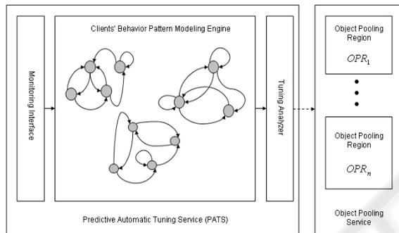
Figure 2: The internal architecture of PATS. Monitoring interface component provides the clients' behavior pattern modeling engine with incoming requests from each client. Then this engine according to the sequences of incoming requests, builds and updates the behavior pattern of each client as a separate markov model. The tuning analyzer component uses these markov models to generate efficient tuning signals which will be sent to the associated object pooling service.
