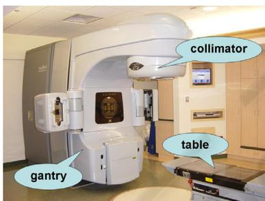
Figure 1: Linear accelerator with on-board imaging.
