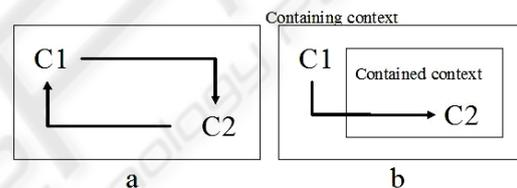
Figure 1: a) developer should avoid logical loops in defining control variables of the same context; b) if C2 is influenced by C1, it should be placed in a context contained by the context that holds C1.
