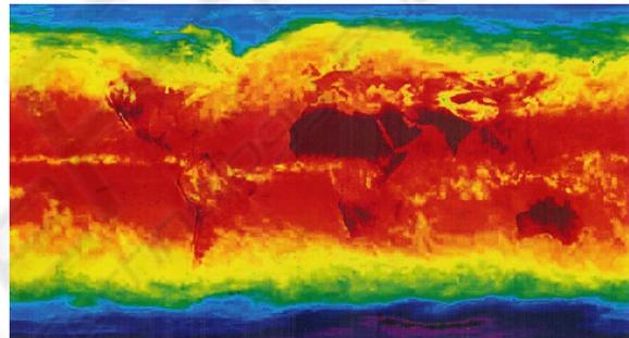
Figure 2: Gridded monthly mean AIRS radiance data, April 2003, from a single window channel at 2616 wave number.
