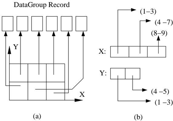
Figure 5: Datagroup array represents the datagroup formed by partitioning the grid array (Figure 4). The index information stores the locations of grid array corresponding to each index value of the respective axis (of datagroup array). A datagroup record stores the list of redundant blocks within each datagroup.
