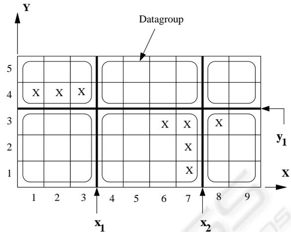
Figure 4: Datagroup formation in a two dimensional grid array. The split locations on  $x$ -axis are  $x_1$  and  $x_2$ , and that on  $y$ -axis is  $y_1$ . The splitting lines are indicated by dark lines. Redundant blocks within a datagroup are indicated by “X” symbol.
