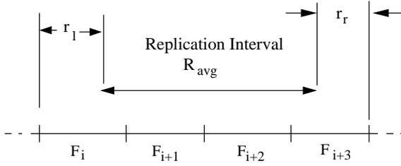
Figure 2: Mapping a replication interval  $R_{avg}$  to fragments where  $r_l$  and  $r_r$  are the redundant intervals. The range of CRS-attribute is represented as the straight line.
