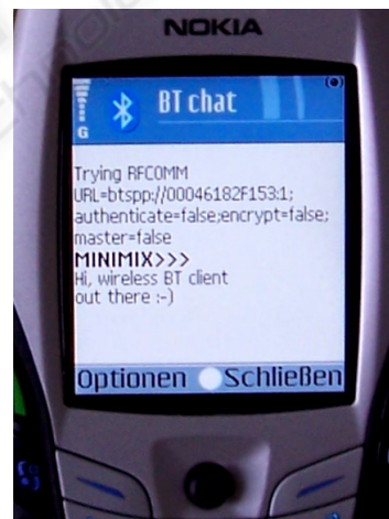
Figure 7: The BT chat client outputs some debug information, before it prints out the input entered on the keyboard of the remotely-connected host MINIMIX.
