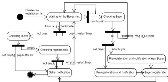
Figure 6: State diagram (Prepare to Negotiation).
