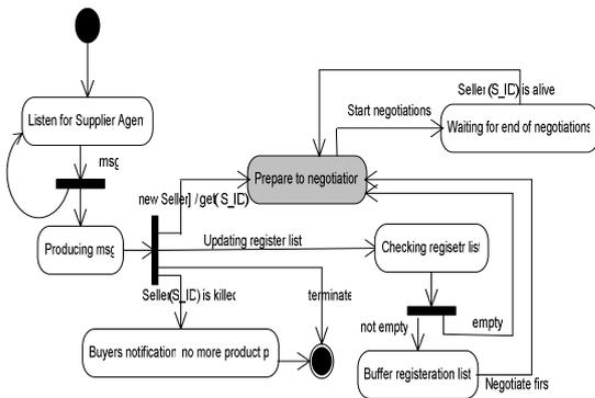
Figure 5: State diagram of the Monitor agent.
