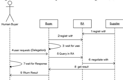
Figure 2: Sequence diagram for system interactions.
