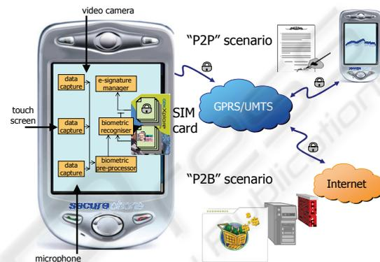
Figure 1: system architecture and service models.
