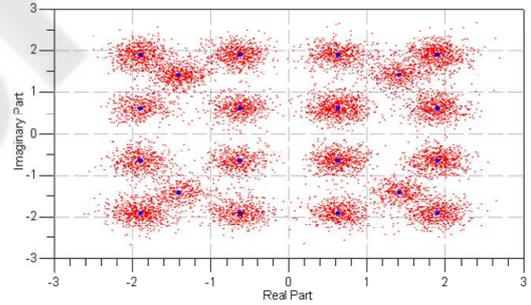
Figure 4: Constellation map of the channel compensated symbols (red) with respect to the transmitted ones (blue).
