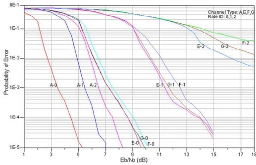
Figure 8: Performance of a  $2 \times 1$  OFDM system in various propagation channels and data rates.
