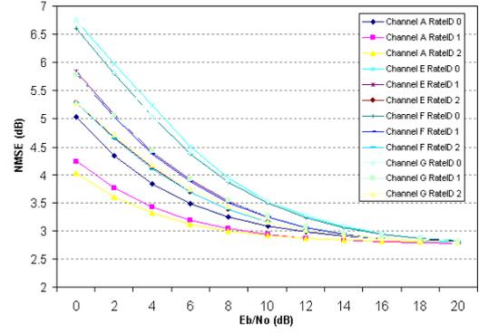
Figure 6: Normalized MSE of the overall channel estimation in various propagation channels and data rates for  $2 \times 2$  MIMO-OFDM case.
