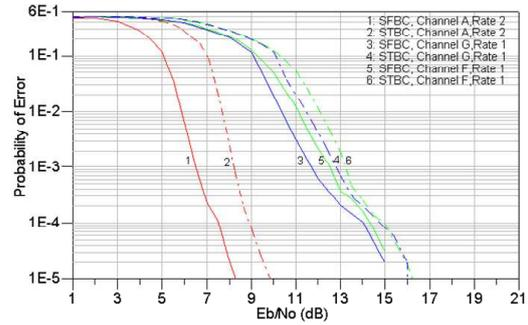
Figure 10: Comparison between SFBC (solid) and STBC (dash) schemes for  $2 \times 1$  case.
