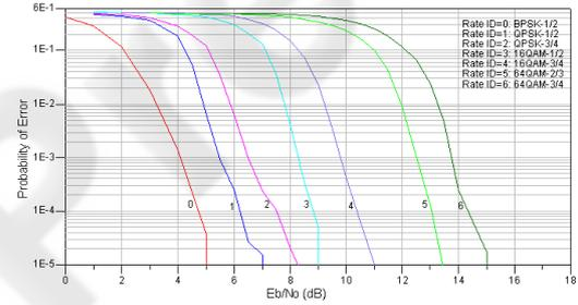
Figure 7: Probability of error for a  $2 \times 1$  OFDM system in propagation channel type A.
