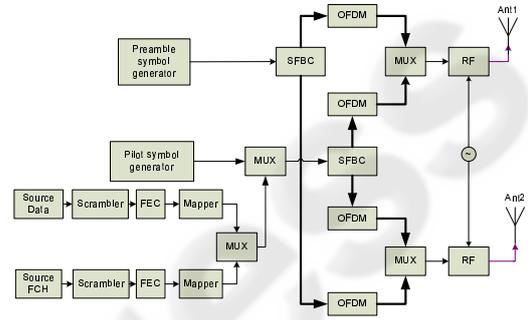
Figure 1: Transmitter Block Diagram.
