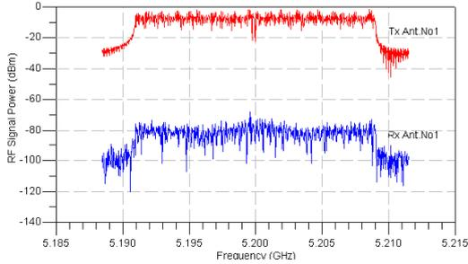
Figure 5: Frequency spectrum at the Tx antenna (red) and the corresponding Rx one (blue) for  $2 \times 2$  OFDM system.
