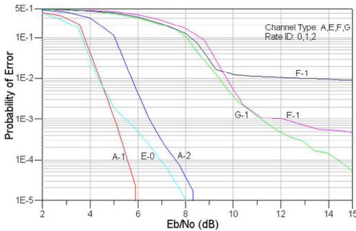
Figure 9: Performance evaluation of a  $2 \times 2$  OFDM system.
