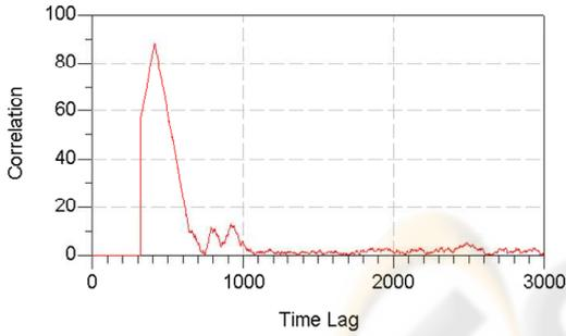
Figure 3: Correlation of time synchronization preamble at the receiver.
