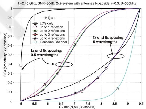
Figure 2: Simulated C-DNFs for different antenna spacings.
