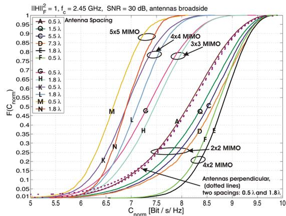
Figure 3: Measured C-CDFs for various settings.
