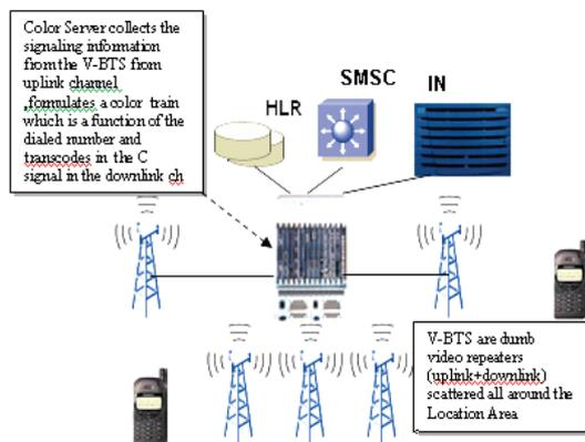
Figure 6: Mobile Network on Colour Signals.
