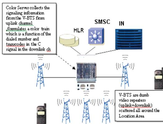
Figure 6: Mobile Network on Colour Signals.
