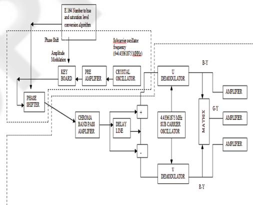
Figure 5: Keyboard Encoder for PCS Mobile Station.
