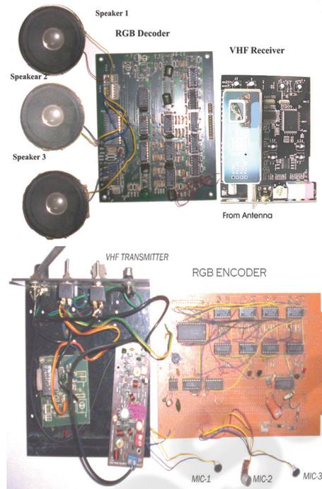
Figure 8: Triple Audio Receiver and Transmitter on Basic Colour Signals (RGB) as carrier signals and built upon PAL VHF Transmitter and Receiver.
