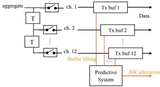
Figure 5: the predictive system scheme. The orange lines indicate the measures used in the predictive system.
