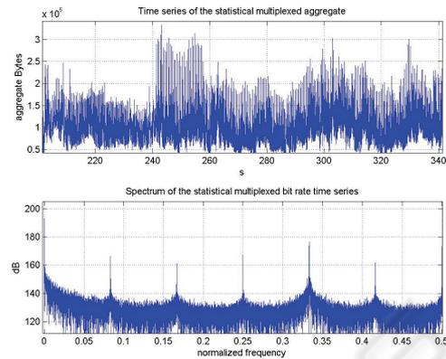
Figure 2: Time evolution and spectrum of a 6 streams CIF aggregate.
