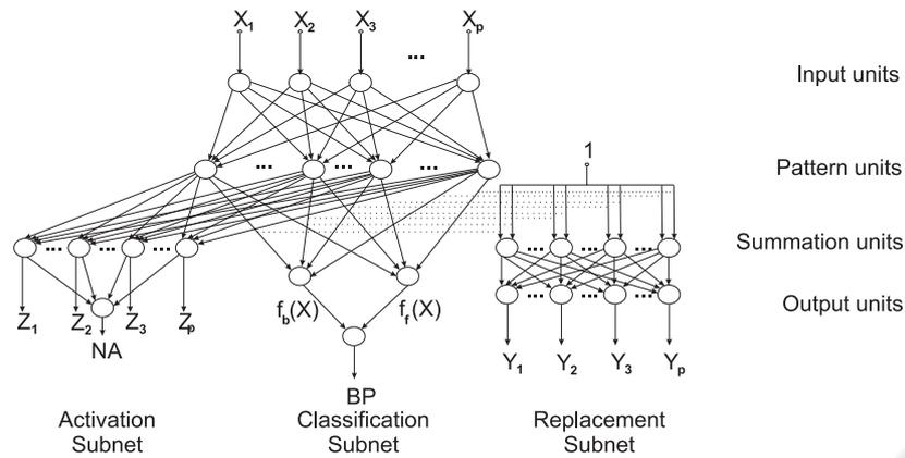
Figure 1: Structure of Background Modeling Neural Network.
