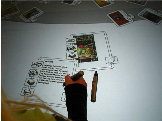
Figure 6: The user interface of the StorySurfer table. Note the high image quality and even light of the low-gain back projection screen.
