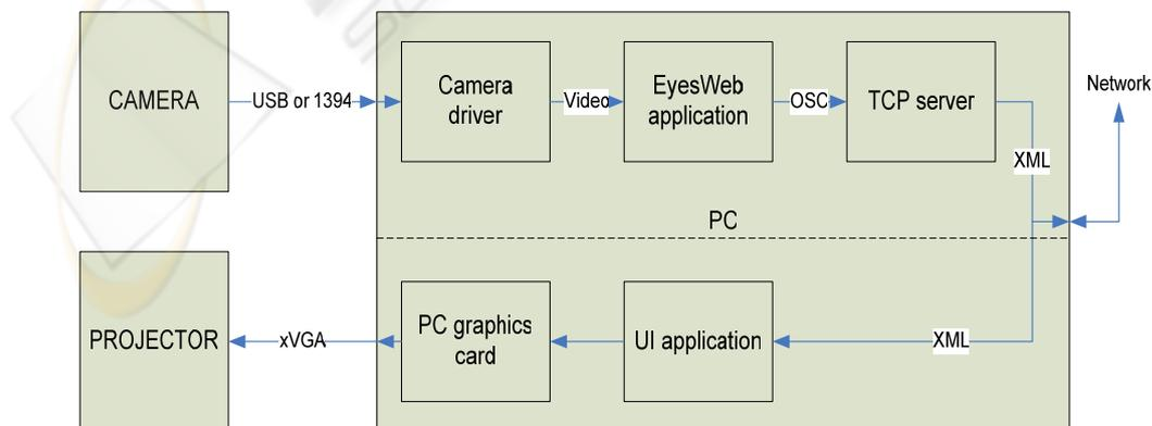
Figure 4: MLT software architecture. The system can run on a single PC if resources allow it, or be distributed on two machines (dashed line).
