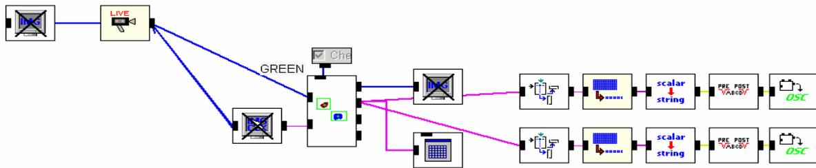
Figure 5: EyesWeb algorithm architecture for tracking a single color.
