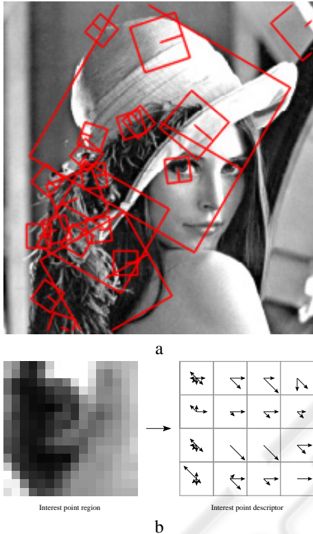
Figure 2: a) Image of Lena with interest points included, the square around each interest point show the size of the descriptor region, and the lines in the squares shows the orientation of the descriptor region. b, left) Detail of the descriptor region for the interest point at Lena's left eye rotated according to the regions orientation. b, right) magnitude and orientation of the 4 \times 4 descriptor histograms. Each of them having 8 directions resulting in 128 entries in the feature vector.
