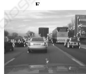
Figure 7: Nonplanarity’ features on first pyramid level of original video-field (cell size  $m_c = 2$ ,  $n_c = 2$ , yielding 125 x 370 cells). Mel size = 2·2 cells; even with these parameters, reducing computing time by more than an order of magnitude, the same image regions with stable features for tracking are found (on larger scales only). [Image compressed 2:1 horizontally after feature extraction.]
