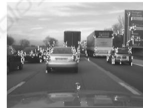
Figure 7: Nonplanarity’ features on first pyramid level of original video-field (cell size  $m_c = 2$ ,  $n_c = 2$ , yielding 125 x 370 cells). Mel size = 2·2 cells; even with these parameters, reducing computing time by more than an order of magnitude, the same image regions with stable features for tracking are found (on larger scales only). [Image compressed 2:1 horizontally after feature extraction.]
