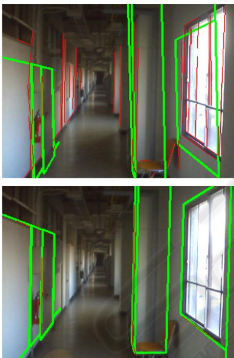
Figure 3: Initial pose and correspondence estimation (Top : Initial guess of the pose and candidates for the corresponding edges, Bottom : Accurately estimated pose and edges corresponding to the line segments of CAD model).
