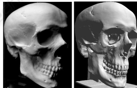
Figure 5: A photograph (left) and the shaded image of the modeled result of a plaster skull (right). Resolutions in rotational direction is 0.02 deg. and in vertical 0.015 mm.
