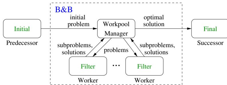
Figure 2: Branch &amp; bound skeleton with centralized work pool manager.
