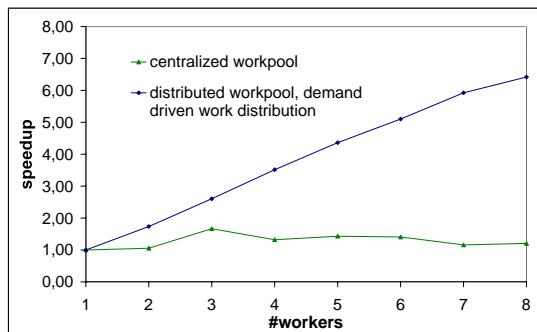
Figure 8: Speedups for 24-puzzle using the central work pool manager and the distributed work pool with demand driven work distribution depending on the number of workers.
