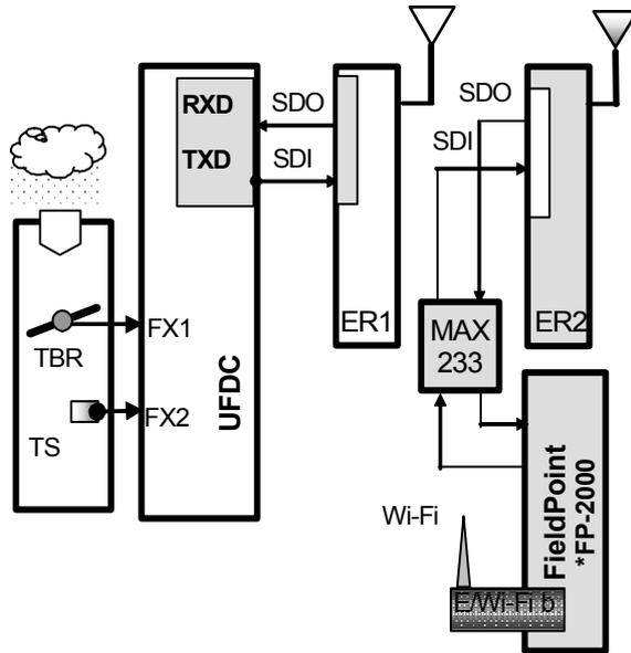
Figure 1: The block diagram rainfall & temperature smart sensing system.
