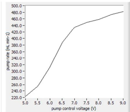
Figure 3: Pump calibration results.
