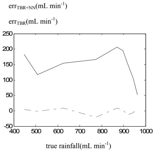
Figure 5: TBR measurement error with and without correction based on neural network.
