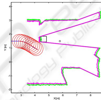
Figure 12c: a new local target was planned and Reactive Simulation computes the trajectory (the red lines). The green line is the received scan and the pink one is the calculated closer scan.
