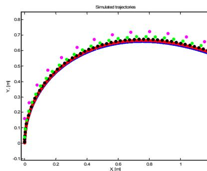
Figure 5: a detail of simulated trajectories with increasing steps of integration: 1 ms (blue), 25 ms (red), 50 ms (black), 100 ms (green), 200 ms (pink).
