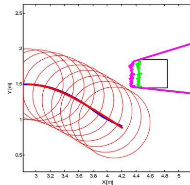
Figure 12d: a detail of Reactive Simulation where the blue line is the real trajectory made by vehicle after the Reactive Simulation.
