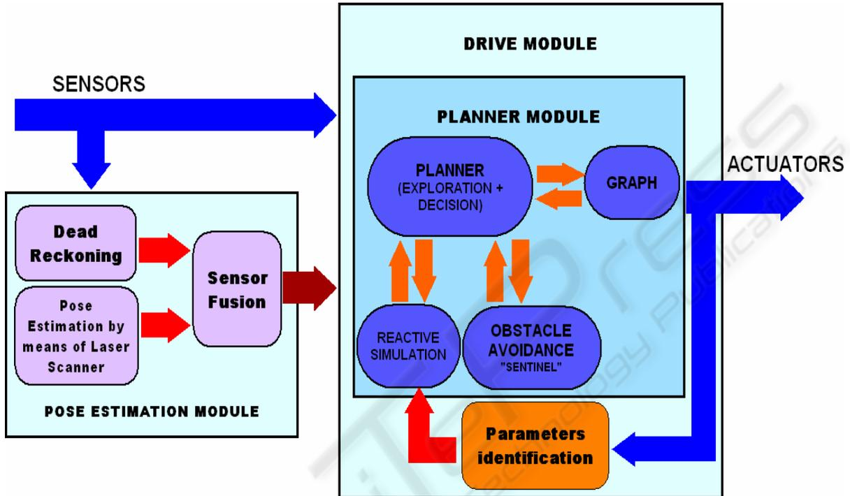
Figure 10: Complete scheme of Drive Module, and its interaction with Sensors Fusion Algorithm and on-line Parameters Identification Algorithm.
