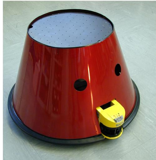
Figure 2: The prototype of AGV used in the experiment.
