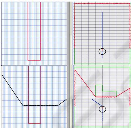
Figure 8a: Example of simulation of obstacle avoidance. On the right side is shown the trajectory of vehicle. On the left side it's shown the Sentinel, which checks a virtual corridor from the actual position of vehicle to the local target to detect any obstacle, as happens in second frame, where an obstacle suddenly appears.
