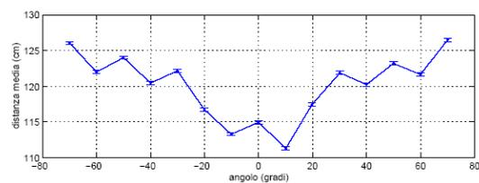
Figure 7: Measurement as a function of the incidence angle. Measurements taken with the target at fixed distance of 115 cm with the apparatus of Figure 6.
