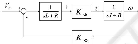
Figure 3: Scheme of CC motor.
