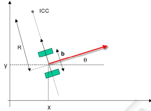
Figure 1: Differential drive kinematics.
