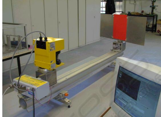
Figure 6: Experimental apparatus used for laser characterisation.
