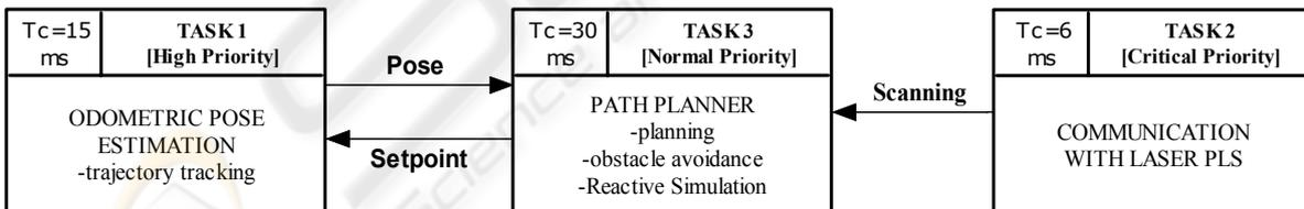
Figure 11: Scheme of the three main tasks.
