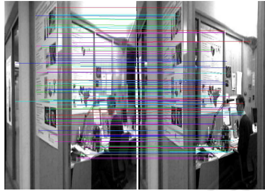
Figure 3: Stereo correspondences using SIFT features. The epipolar constrain is used to find correspondences across images.
