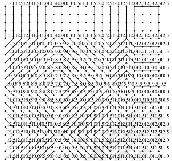
Figure 5: The functional relief of the bidimensional interconnection with elementary structures  $EIS4$  and  $EIS5$  for uniform distribution. The contour patterns of the functional average distance  $\bar{d}_U(O)$  are drawn.
