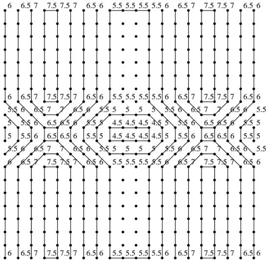
Figure 4: The functional relief for the bidimensional non-homogenous interconnection with the elementary structures  $EIS2$  and  $EIS3$ . The contour patterns of the functional average distance  $\bar{d}_U(O)$  for the uniform distribution are drawn.
