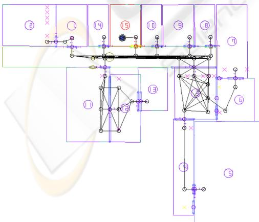
Figure 9: Autonomously explored simulated environment with navigation graph.
