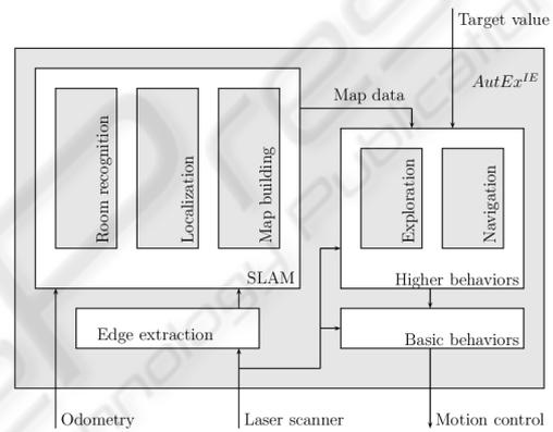
Figure 5: Exploration structure of the robot Marvin.
