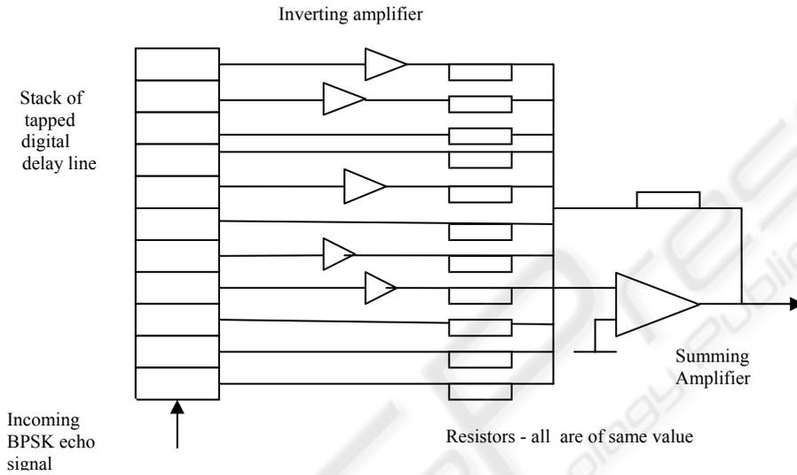
Figure 4: Replica Correlator Circuit.
