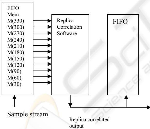
Figure 8: Flow of data stream for replica correlation.
