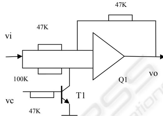
Figure 7: Controlled inverter circuit.
