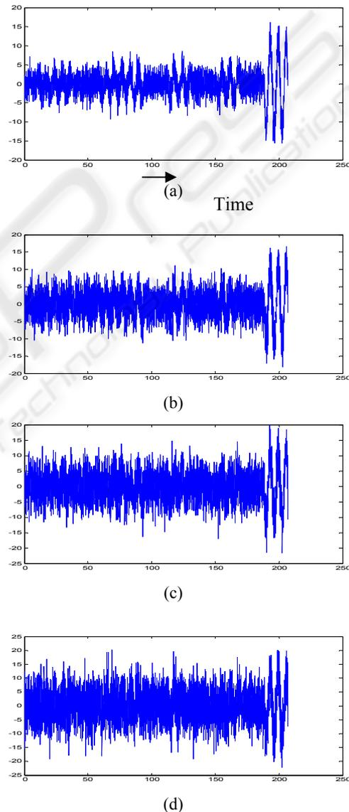
Figure 9: Replica correlated output ; Amplitude vs time for one packet duration. a. 200% noise b.300% c.400% d.500%.
