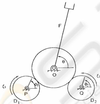
Figure 2: One-DOF Mechanism with redundant unidirectional drives.
