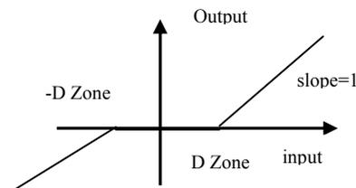
Figure 6: Input-output characteristic curve for deadzone nonlinearity.
