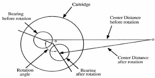
Figure 1: Backlash control mechanism using adjustable centre distance.
