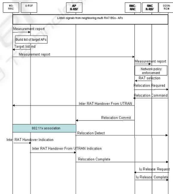
Figure 4: Handing over a connection from UTRAN to WLAN
