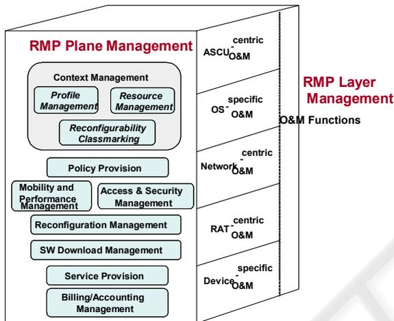
Figure 1: The reconfiguration management plane.
