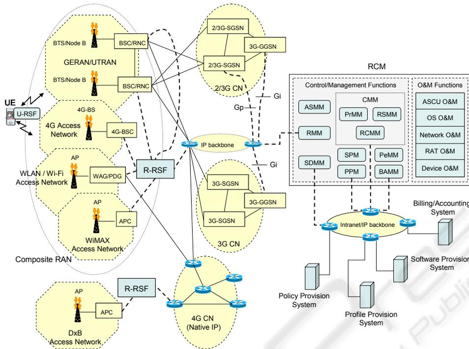
Figure 1. The RMP in a Beyond 3G mobile network architecture.
