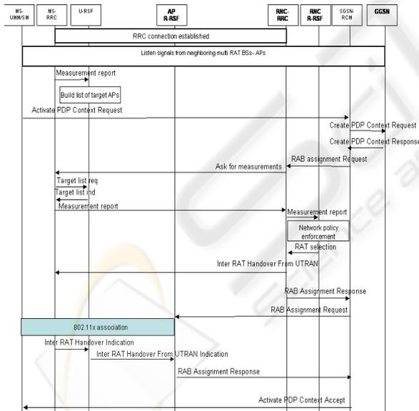
Figure 3. Outgoing connection setup through WLAN
