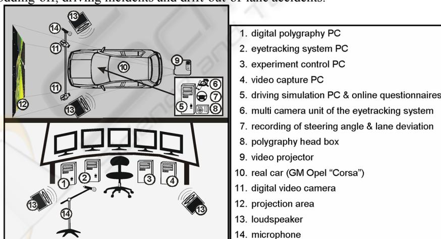
Fig. 1. Real car driving simulation laboratory
