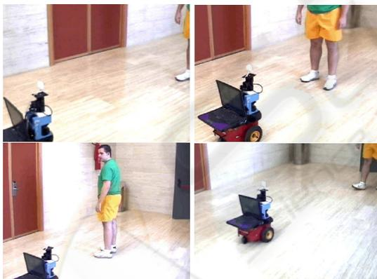
Figure 7: Robot keeps the distance using only vision
