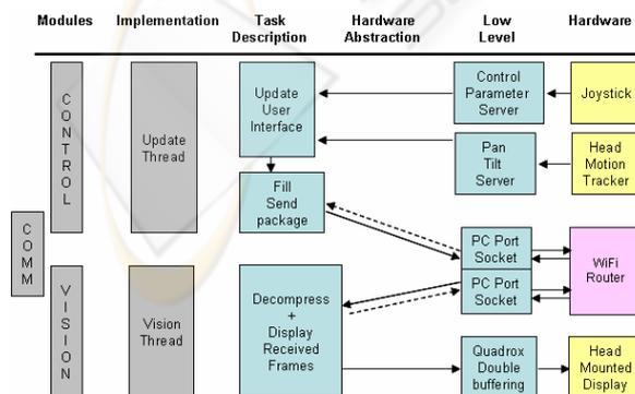
Figure 2: Client or operator system architecture
