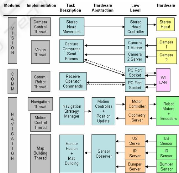
Figure 1: Robot system architecture
