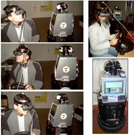
Figure 3: The Nomad200 robot with the upper PC-platform and the biclops head on top. The stereo vision system forms the robot's eyes
