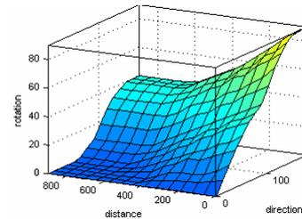
Figure 6: Transfer function of the controller for Goal seeking
