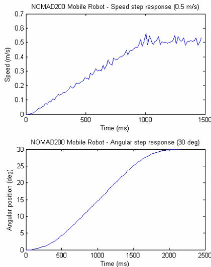
Figure 8: Speed and angular step response from the Nomad200 robot platform
