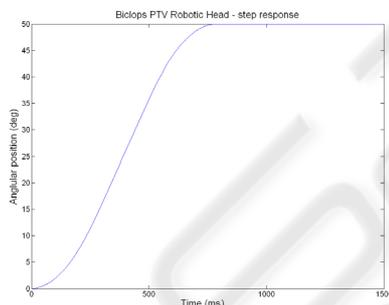
Figure 9: Biclops robotic head step response
