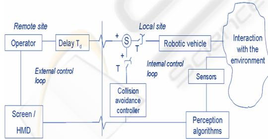
Figure 5: Obstacle avoidance control architecture.
