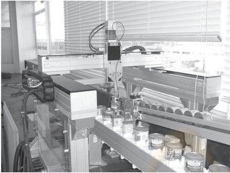
Figure 2: Gantry robot, conveyor and payload dispenser
