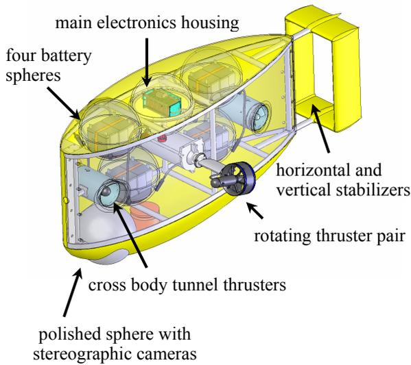
Figure 3: Simplified view illustrating the major components of the Odyssey IV design
