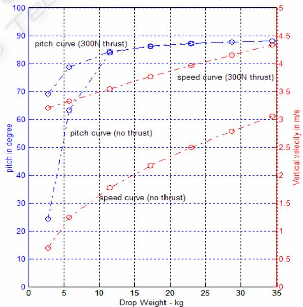
Figure 4: Descent speed and pitch angle as a function of drop weight mass. The weight is placed at the nose to cause the body to pitch down to present a more streamlined axis to the flow. The lift on the rear stabilizers cause the body to pitch further nose down, increasing the speed and stability of the dive.
