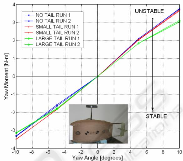
Figure 5: Yaw moment as a function of yaw angle for a series of tail sizes. These results indicate that the tails used for these test have insufficient area to make the body passively stable. In order to achieve passive stability, the rear vertical stabilizer will need to have at least 400% more area. A new model tail is being constructed, and another series of tests will be performed to verify that the increased tail area will enable the body to be passively stable in tow
