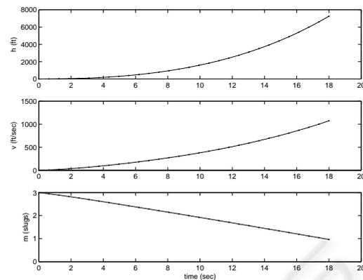
Figure 4: The state variables, the altitude, velocity and mass of the rocket as a function of time
