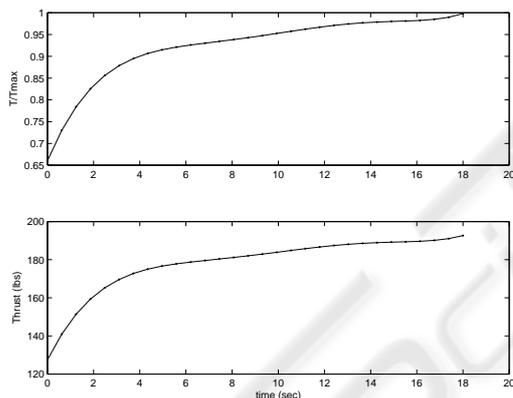
Figure 3: The thrust control history. The upper graph displays the value of the thrust normalized by maximum thrust. The lower graph shows the actual thrust in lbs.
