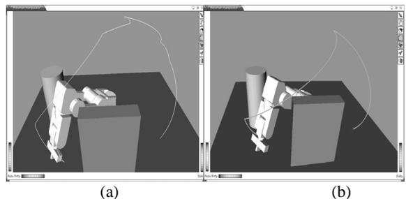
Figure 4: (a) raw trajectory, (b) Euclidian norm A\* path.
