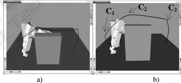
Figure 7: a) cutting-triangle-edge path: b) cubic smoothing path.
