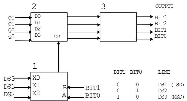
Figure 3: Interface module for connection of an ultrasonic ranging system *POLAROID* to an external microprocessor system: block diagram
