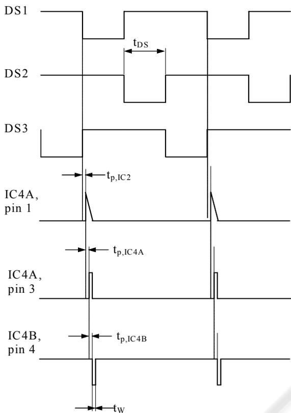
Figure 5: Interface module for connection of an ultrasonic ranging system POLAROID to an external microprocessor system: timing diagram
