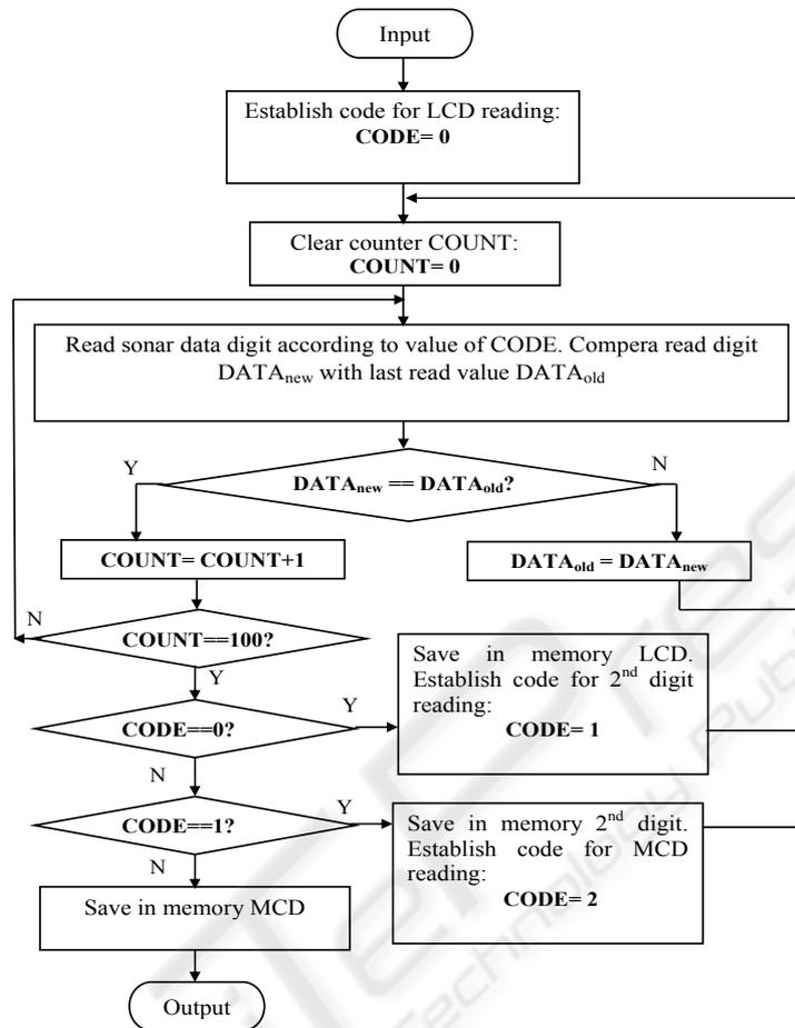
Figure 6: The algorithm of the software filter.
