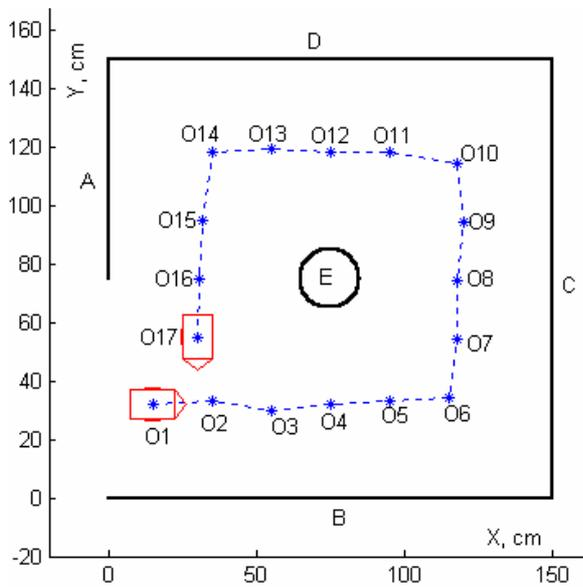
Figure 7: Gleaning of information from environment by moving mobile robot and scanning ultrasonic range finder: experimental laboratory environment and robot path.
