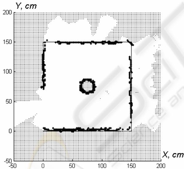
Figure 8: An experimentally obtained integrated occupancy grid map of the environment, represented in Figure 7. The empty cells are leaved by white; thick black crosses label the occupied cells; and small points label the indeterminate cells.
