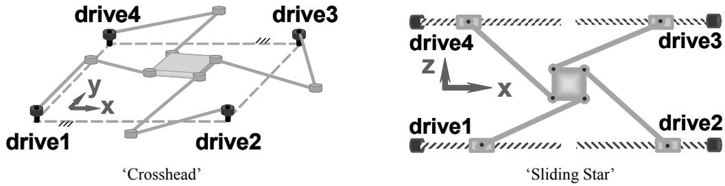
Figure 1: Planar parallel robots: horizontal and vertical
