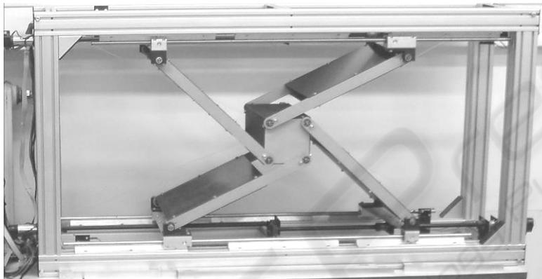
Figure 3: Lab model of parallel robot ‘Sliding Star’
