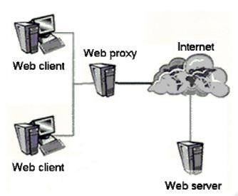
Figure 1: Web proxy in network configuration.
