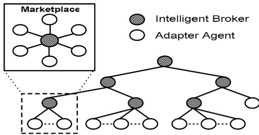
Figure 2: Hierarchical Broker Framework
