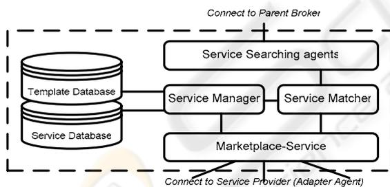
Figure 5: Intelligent Broker Architecture
