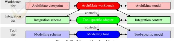
Figure 2: The 3-tier workbench architecture
