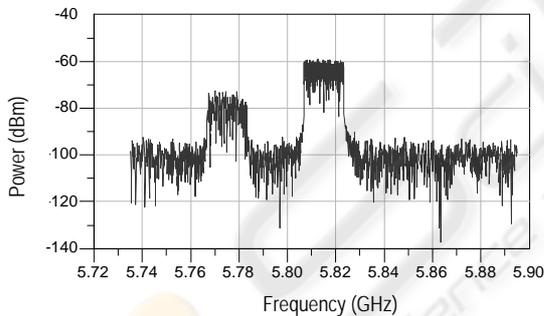
Figure 4: Alternate Channel Rejection
