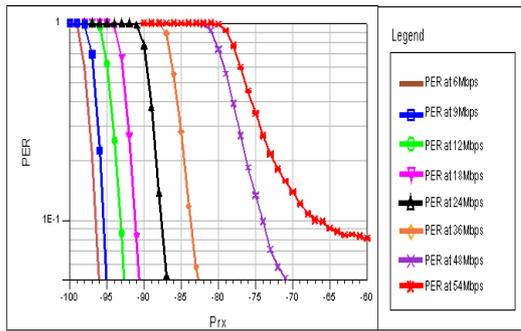
Figure 2: Receiver Sensitivity
