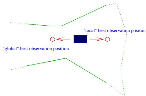
Figure 10: Greedy selection of candidates, dashed lines are walls not yet perceived by the robot
