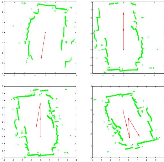
Figure 5: A sequence of observation positions reached by the robot with  $r_{max} = 4$  m
