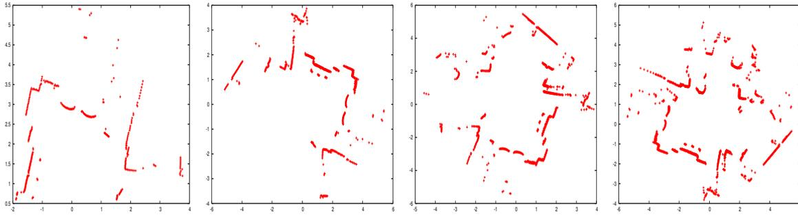
Figure 1: The construction of a partial map of a scattered environment obtained by aligning four scans (points of the map are represented as crosses, the current position of the robot is  $(0, 0)$ , scales are in meters)
