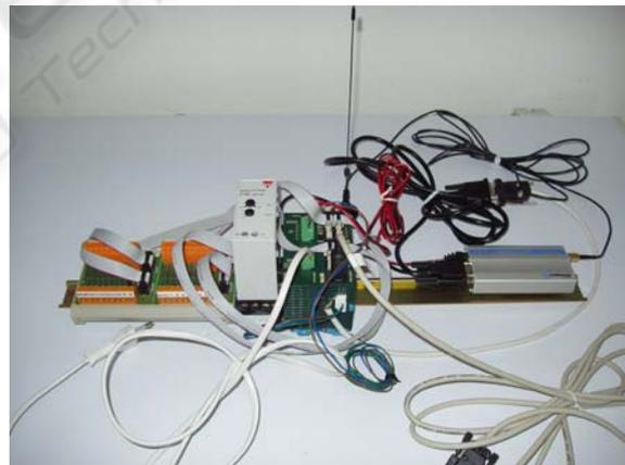
Figure 3: Photo of the implemented remote station prototype.
