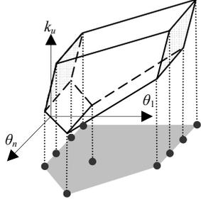
Figure 2: The polyhedral domain and its projection on the context parameters subspace.
