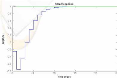
Figure 5: Open loop step response.
