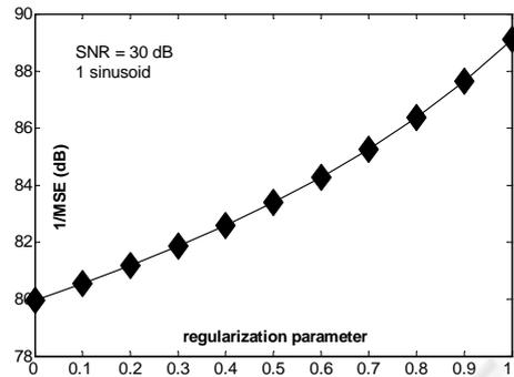
Figure 7: Estimation results obtained from the Smyth algorithm and the regularization procedure as a function of the regularization parameter: SNR: 30 dB.
