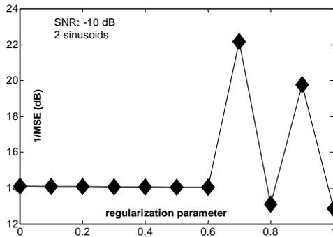
Figure 5: Estimation results obtained from the Smyth algorithm and the regularization procedure as a function of the regularization parameter: SNR: -10 dB.
