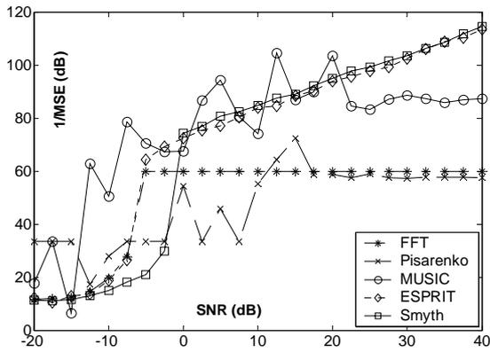
Figure 1: Performance results from pseudo Monte Carlo analysis for the estimation of a single frequency. dash-dot line: FFT; dashed, with crosses: Pisarenko; continuous line, with circles: MUSIC; dotted line, with diamonds: ESPRIT; continuous line with squares: Smyth.
