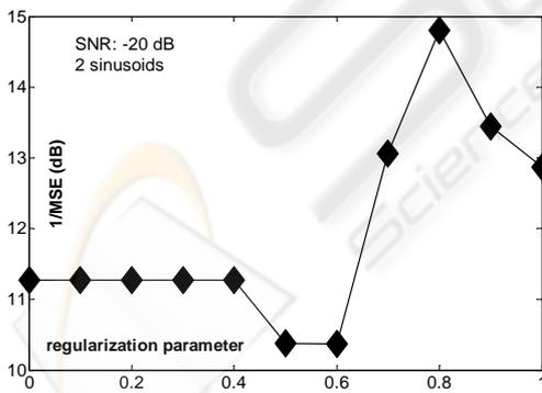
Figure 6: Estimation results obtained from the Smyth algorithm and the regularization procedure as a function of the regularization parameter: SNR: -20 dB
