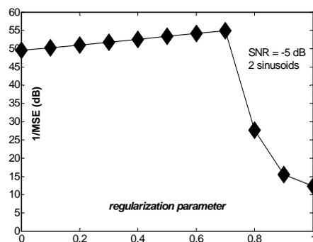
Figure 4: Estimation results obtained from the Smyth algorithm and the regularization procedure as a function of the regularization parameter; SNR: -5 dB.
