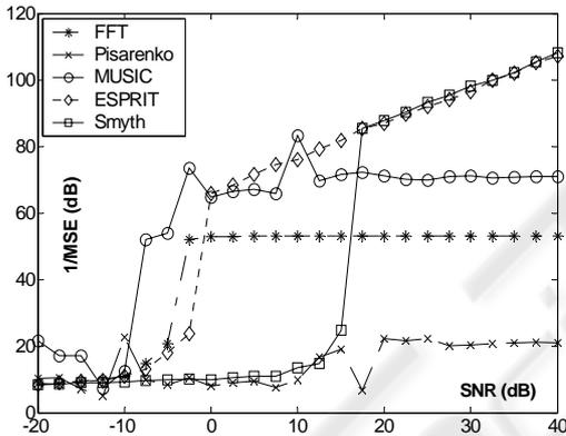
Figure 2: Performance results from pseudo Monte Carlo analysis for the simultaneous estimation of two frequencies; dash-dot line: FFT; dashed, with crosses: Pisarenko; continuous line, with circles: MUSIC; dotted line, with diamonds: ESPRIT; continuous line with squares: Smyth.
