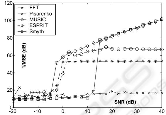
Figure 3: Performance results from pseudo Monte Carlo analysis for the simultaneous estimation of four frequencies. dash-dot line: FFT; dashed, with crosses: Pisarenko; continuous line, with circles: MUSIC; dotted line, with diamonds: ESPRIT; continuous line with squares: Smyth.
