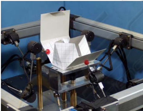
(c) Folding motion for "Boy-scouts tent" type carton box Figure 8: The test motion of a carton flap folding
