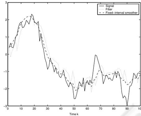
Figure 2: Signal, filtering and fixed-interval smoothing estimates for  $p = 0.1$ .
