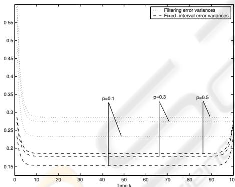
Figure 1: Filtering and fixed-interval smoothing error variances for  $p = 0.1, 0.3, 0.5$ .
