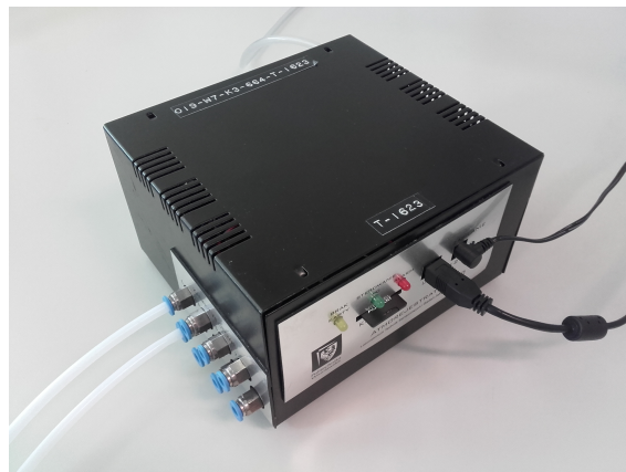
Figure 1: Sensor System with Multi-point Sampling in Technical Space.
