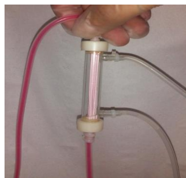
Photo 1: The module with asymmetric capillaries made of polysulfone with a 10 kDa cut-off point (IBIB-PAN, Warsaw).
